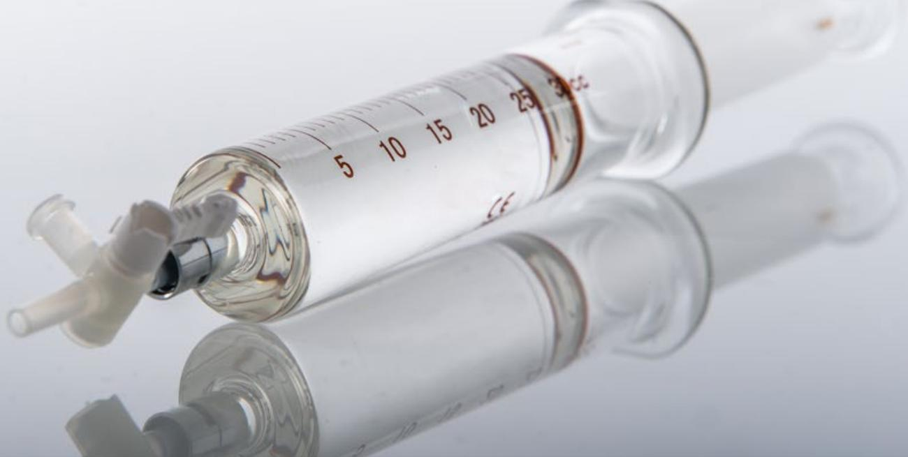
**True North gas-in-oil standards** ensure proper calibration of gas extraction and chromatography
